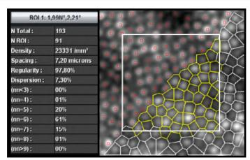
Example of analysis results in metric units. Visual units are also available for reduced variability in Voronoi cell density and inter-cell spacing<sup>[2]</sup>.
